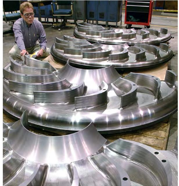
Our compressors use either fabricated steel diaphragms or a combination cast-and-fabricated steel design, where thickness precludes using steel plate alone. Precision machining ensures dimensional accuracy and significantly improves the diaphragm surface finish. Diaphragms are horizontally split and finished at all horizontal and peripheral joints and on gas path surfaces.
