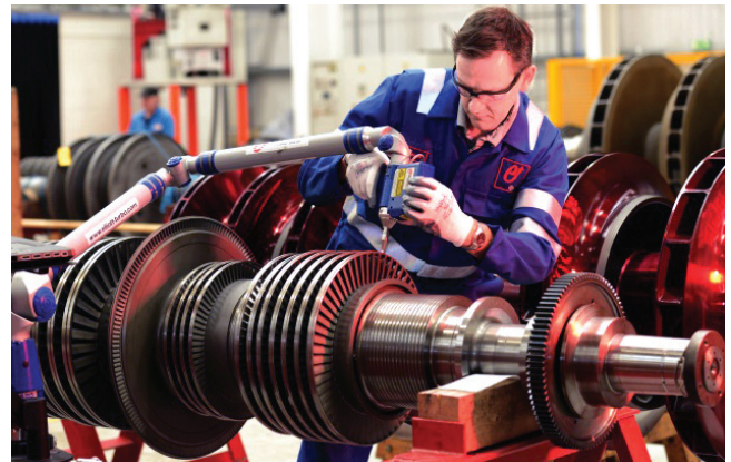
Reverse engineering of a non-Elliott steam turbine rotor using CMM.
