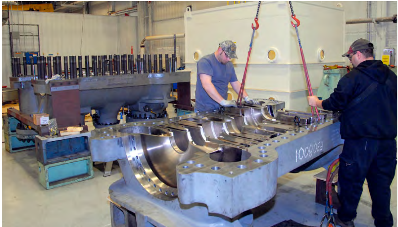
Assembly of a drop-in replacement for a 30-year old compressor. Design enhancements for this machine included solid end walls, abrasable seals, and improved diaphragm and impeller materials.
