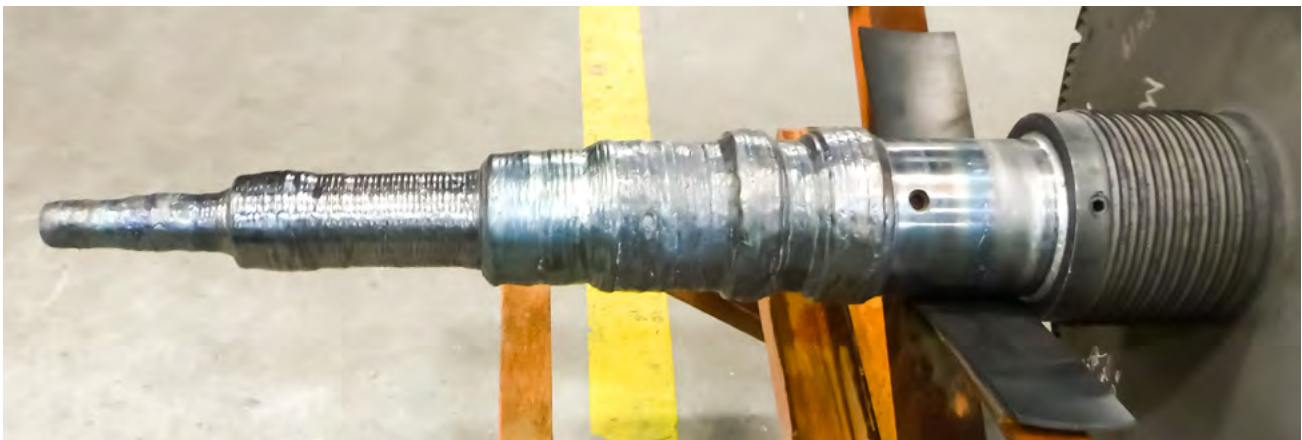
Sub-arc welding process – weld buildup on rotor prior to machining.
