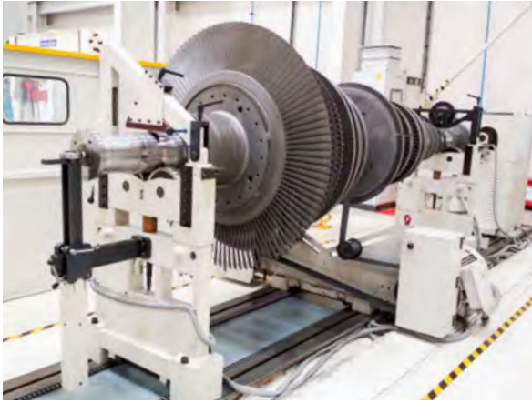
Rotor in balance machine.
