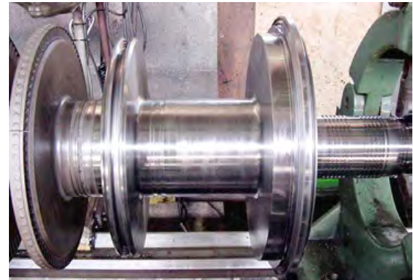
Repaired disk with machined slots.
