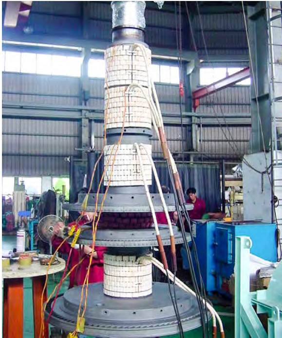
Shaft undergoing stress relief for straightening.
