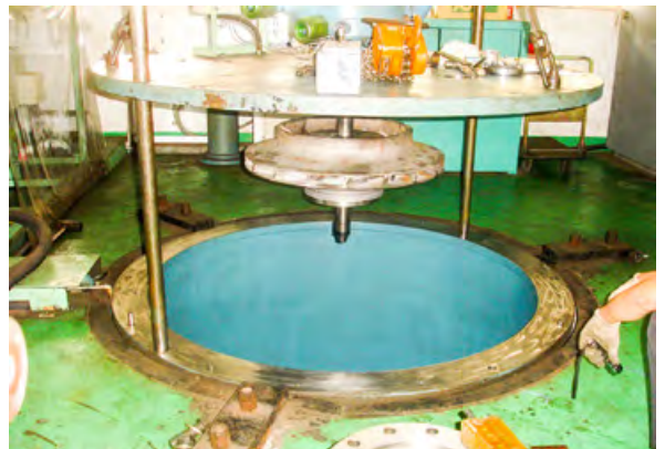
Spin pit for spin testing.
