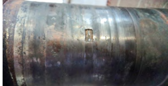
Damaged packing area.
