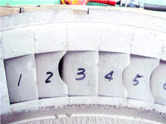
Damaged stator blade.
