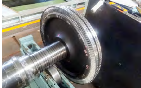
Installing shroud rings.
