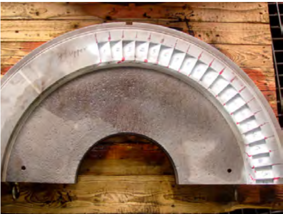
Nondestructive testing after repair.
