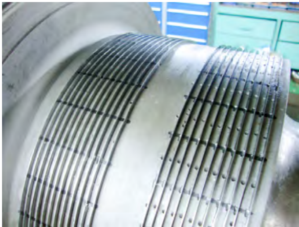
New sealing strip.
