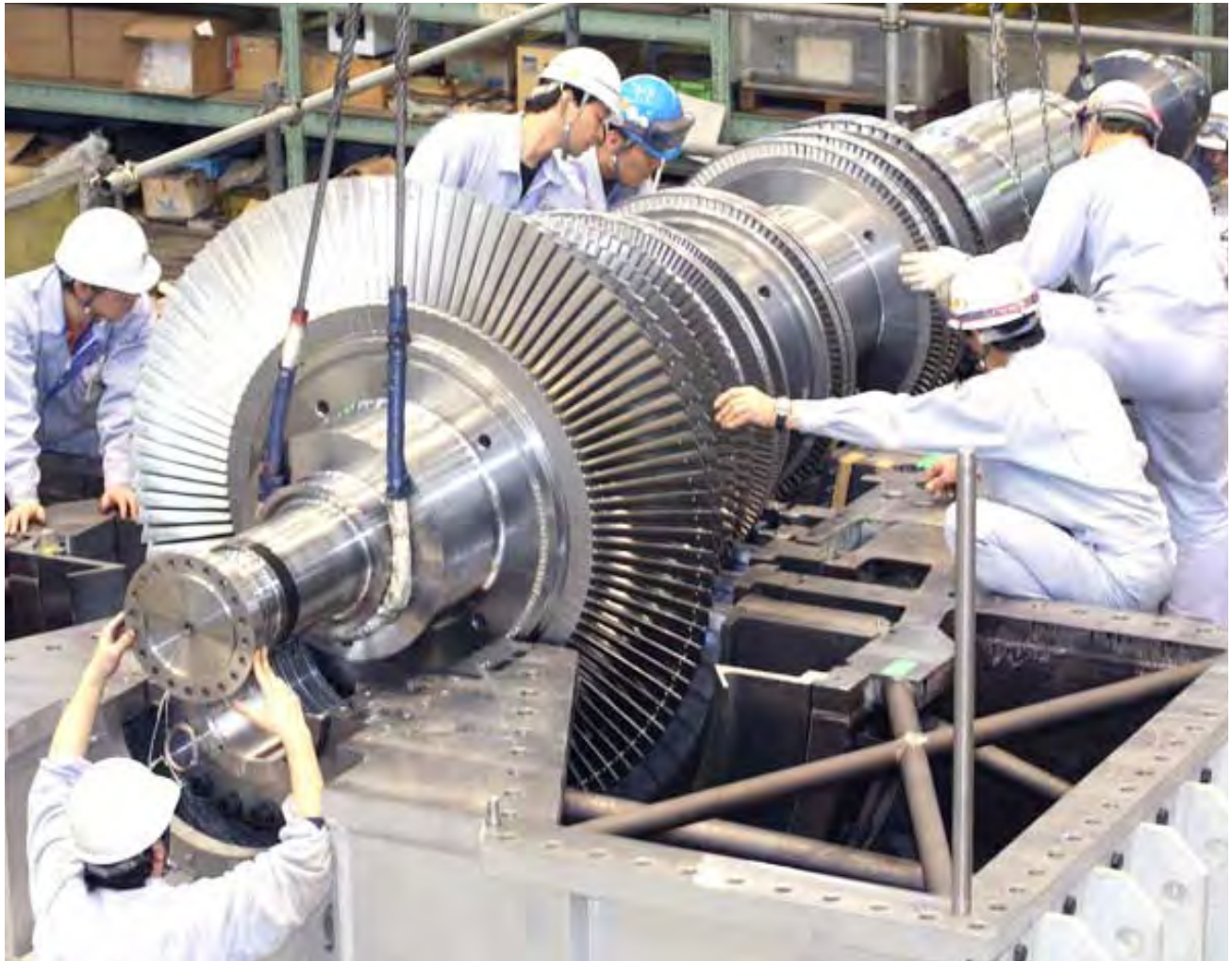
Multi-stage, multi-valve steam turbine assembly.
