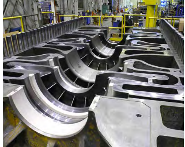
88M6-4 refrigeration compressor with two side loads.
