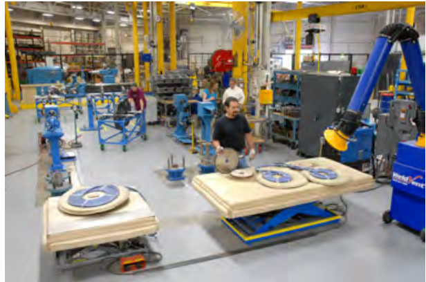
Induction heating of rotor disks speeds the assembly of YR turbine rotors.
