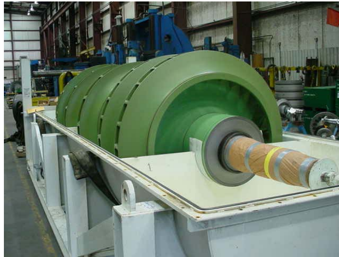
Figure 2. Centrifugal Compressor Rotor Coated with a PTFE Type Coating.
