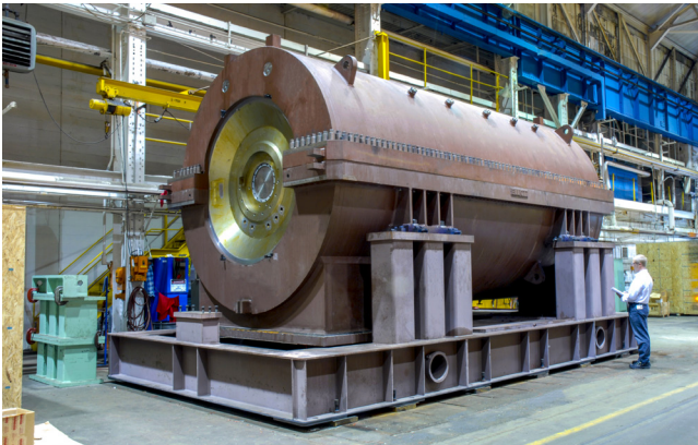
Figure 2. An Elliott 110M compressor during manufacturing.
