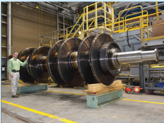
Large compressor rotors, diaphragms and casings are manufactured, balanced and tested on site
