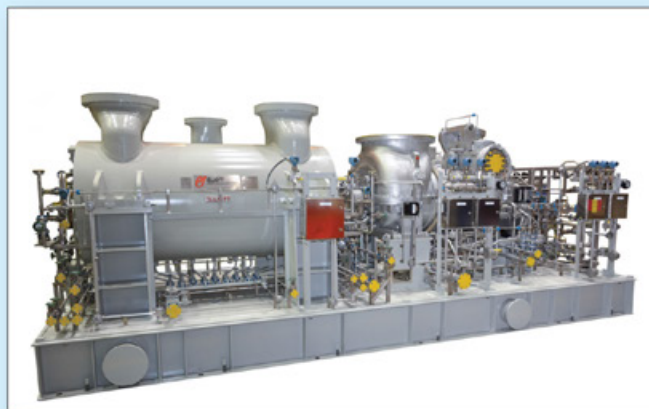
Steam turbine-driven mixed refrigerant compressor trains are produced by Elliott
