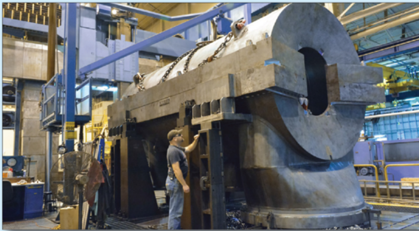
Massive casings like these are cut, machined, welded and finished in the Elliott facility
