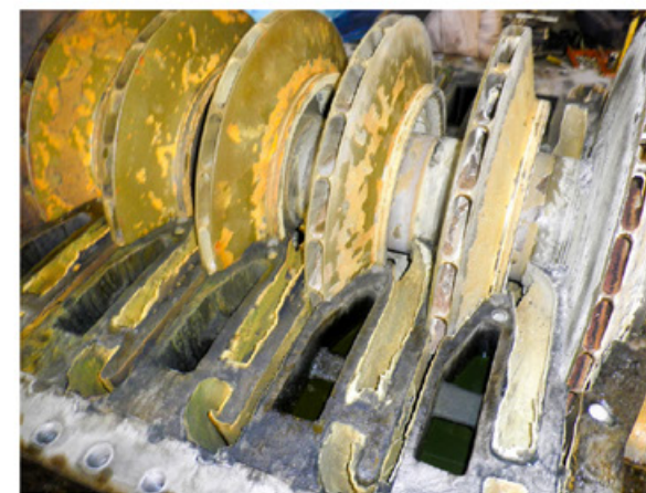
Figure 3. A H 2 recycle compressor with chloride fouling.
