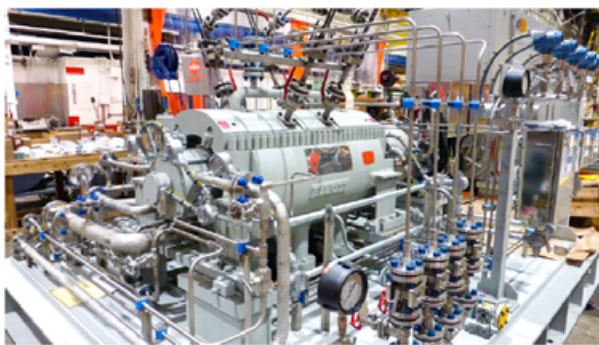
Figure 5. Compressor with a removable wash system.
