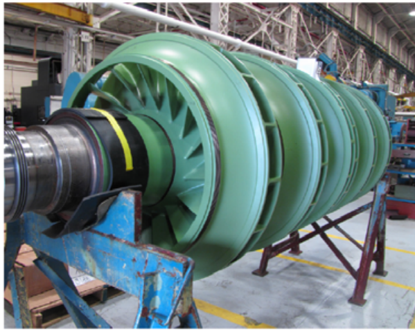
Figure 4. Compressor rotor with protective coating.
