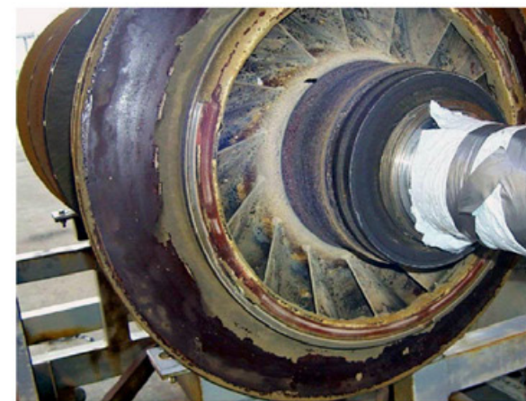
Figure 2. A charge gas compressor with erosion damage.
