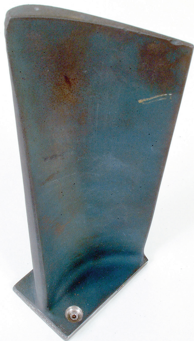
Figure 2. Elliott TH-100 expander blade after nine years of continuous operation.
