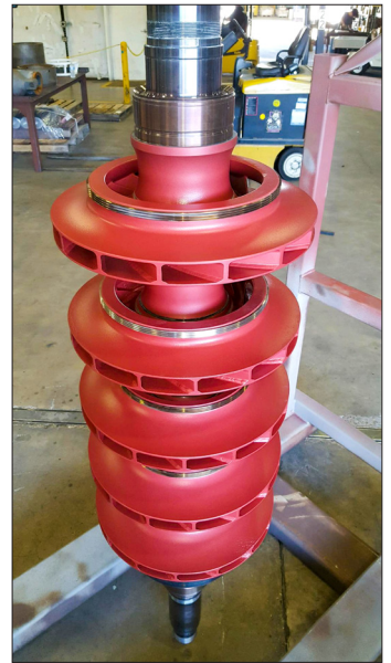
Figure 2: A specialty hydrogen recycle coating developed by Elliott was applied to a 5-stage compressor rotor in hydrogen service. Its anti-fouling properties prevent buildup of material in the gas path, provide corrosion resistance against ammonium chloride, and increase wear and durability resistance to solid particle erosion. It is good for continuous operation up to 500°F (260°C).
