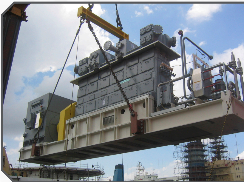
Mitsubishi Heavy Industries: MHI's LNG Refrigeration Compressor performance testing before site installation.
