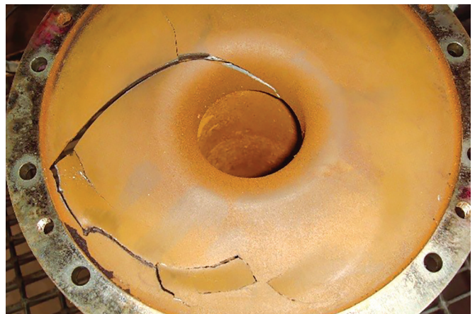
FIG. 1. Failed diaphragm coupling.
