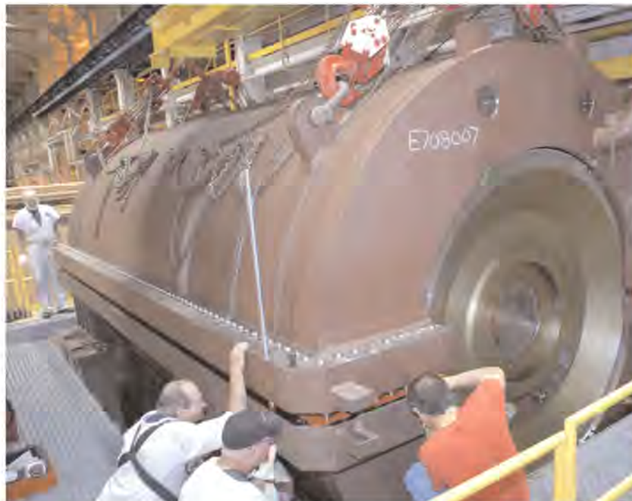
Figure 1: The Elliott 110M Compressor consists of a single casing that supports a rotor of nearly 24.5 ft length. The machine acts as booster compressor from the propylene reactor to the compressor trains at the Houston facility
