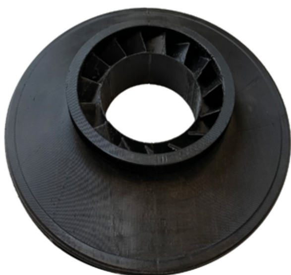
Figure 2. Elliott is evaluating non-metallic impellers for compression applications such as the use of directionally wound carbon fibre impellers.
