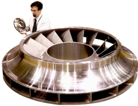
Figure 3. The use of advanced aerodynamic and structural design/analysis tools make the development of highly efficient compressors for hydrogen, carbon dioxide, and natural gas possible.
