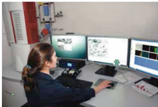
Figure 5. Materials engineer using the SEM to examine material microstructure and composition.
