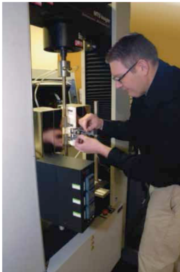
Figure 4. Materials engineer arranging a stress relaxation test specimen.
