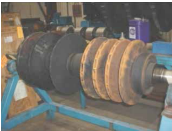
Figure 2. Compressor rotor with extensive corrosion.
