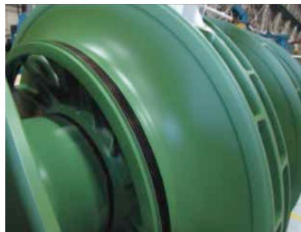
Figure 3. Compressor rotor coated with Pos-E-Coat Plus.
