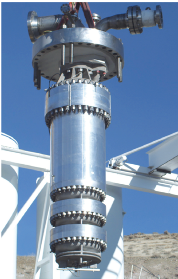
Figure 4. A cryogenic liquid expander on test at the Cryodynamics facility in Sparks, Nevada, USA.
