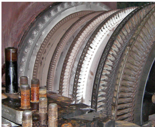
Figure 1. Turbine rotor with mineral deposits.
