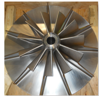
New one-piece impeller manufactured at the Elliott Jeannette, PA facility.
