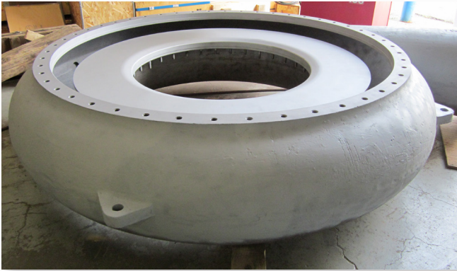
Refurbished casing after hydrotest and blast cleaning.
