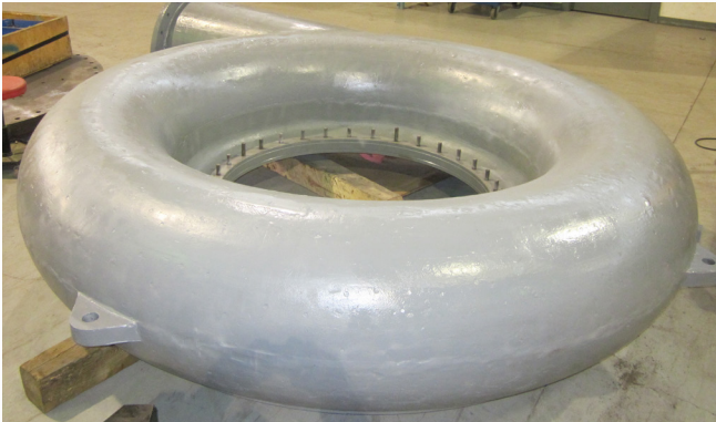
Painted casing ready for final assembly.
