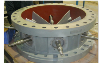
Refurbished inlet guide vanes.
