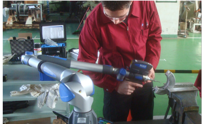
Elliott engineer measuring a journal bearing with a portable CMM and hand-held scanner.
