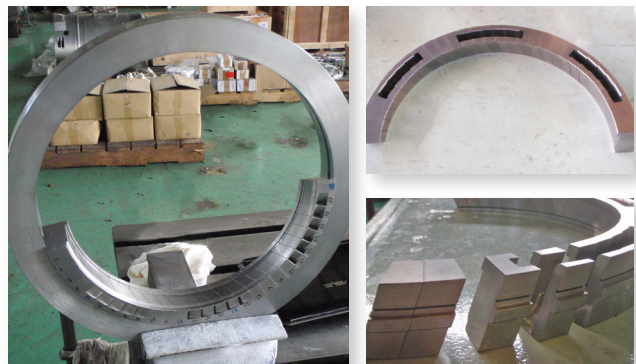
Typical nozzle rings are one piece. The nozzle ring in the refinery's diesel unit's steam turbine was comprised of individual segments that fit into a channel, making it difficult to measure. Elliott manufactured the fixture pictured on the left to hold the nozzle segments in their arc formation for accurate measurement.
